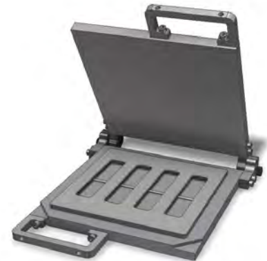
Mould for Samples for Flex Testing
